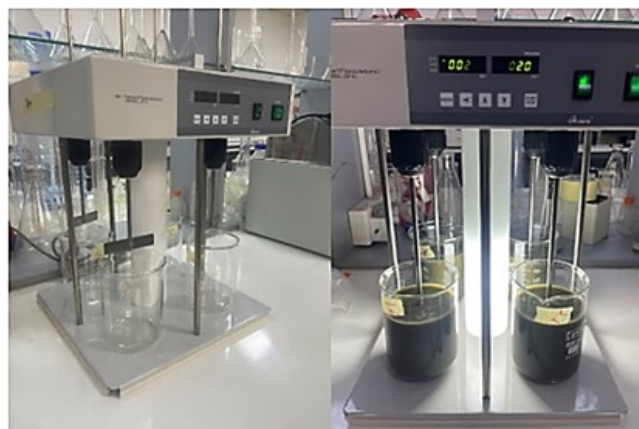
Figure 1. Jar test used in the coagulation and filtration of DCFW
