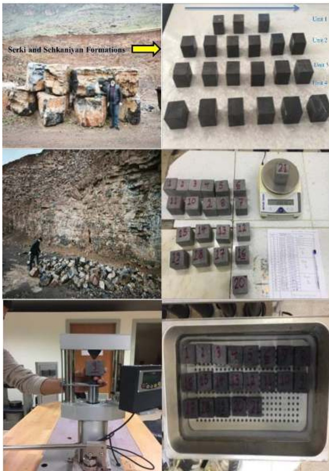
Figure 3. Rock sample collection, cutting, dry and wet weighting and point load testing.
